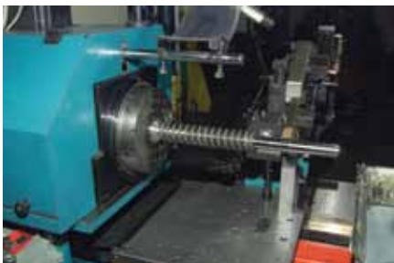
Coilers - Using the latest in CNC coiling technology, springs are produced with much better predictability and consistency in performance, rates and lengths.
