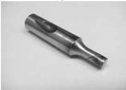
• Excessive heat due to tight clearance
