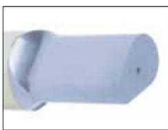
**TiCN (XCN)**—ultra-hard (harder than carbide), thin PVD coating. Provides superior abrasive wear resistance and lubricity. Well-suited for stainless steel, nickel, and copper. Approx. hardness: \*Vickers 3000.
