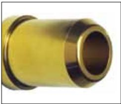
**DayTiN® (XNT)**—PVD coating provides excellent wear resistance and lubricity. Not recommended for stainless steel, copper, or nickel. A good general-purpose coating. Approx. hardness: \*Vickers 2300.
