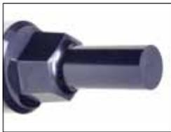
**DayTAN™ (XAN)**—ultra-hard (harder than carbide), high-aluminum PVD coating. Provides high temperature resistance. Well-suited for applications where surface heat is generated. Ideal for HSLA, dual phase, and TRIP steels. Approx. hardness: \*Vickers 3400.
