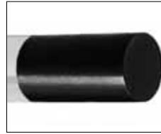
**XCD**—diamond-like carbon coating. Combines high hardness with an extremely low coefficient of friction. Good protection against abrasive and adhesive wear. Ideal for aluminum. Approx. hardness: \*Vickers 2500.
