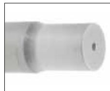
**CRN**—excellent adhesion, high toughness, and good corrosion resistance. Primary applications are metal forming (copper, brass, & bronze), metal die casting, and plastic injection molding. Approx. hardness: \*Vickers 1800-2100.
