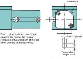
The air cylinder can be removed and remounted 90° or 180° from the location shown.
