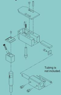
The BRAR Reversible Change Retainers come complete with all the necessary screws, dowels, the air cylinder, lead wires, the autoswitch, and the fittings.
